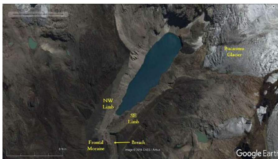
Figure 4. Lake Palcacocha, at the northeastern end of the Cojup Valley with the Pucaranra Glacier lying to the northeast. The breach in the frontal moraine is the result of the 1941 outburst flood. Image source: Google Earth, 2018.
